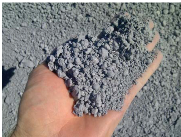
Figure 5. Metallic aluminium residue from the mill.
