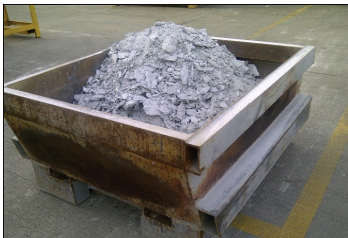
Figure 3. Skip of SRSS residue ready to be fed into the Phase I Bath Plant Facility.
